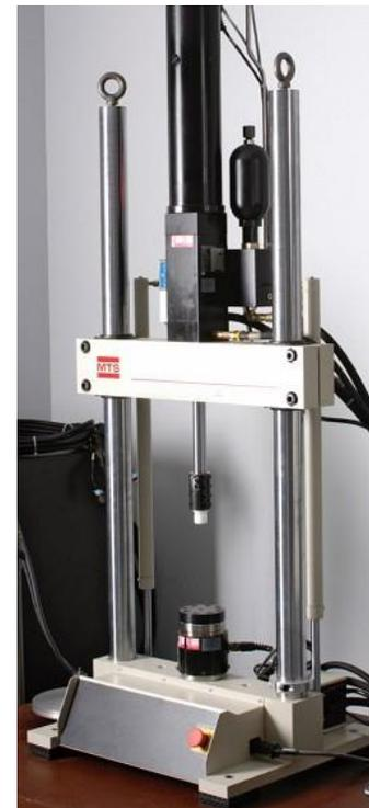
MTS Bionix Axial Torsion System
